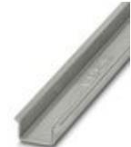
DIN rail, unperforated, Standard profile 2.3 mm, width: 35 mm, height: 15 mm, acc. to EN 60715, material: Steel, galvanized, passivated with a thick layer, length: 2000 mm, color: silver
