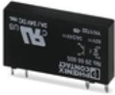
Plug-in miniature solid-state relay, power solid-state relay, 1 N/O contact, input: 60 V DC, output: 3 ... 33 V DC/3 A
