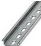
DIN rail perforated, Standard profile, width: 35 mm, height: 7.5 mm, acc. to EN 60715, material: Steel, galvanized, length: 2000 mm, color: silver
