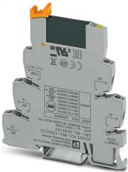
PLC-INTERFACE, consisting of PLC-BSC.../21 basic terminal block with screw connection and plug-in miniature solid-state relay, for mounting on DIN rail NS 35/7,5, 1 N/O contact, input: 120 V AC/110 V DC, output: 3 - 33 V DC/3 A
